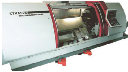
CNC-Turning up to 4 axes and up to 2.000 mm distance
