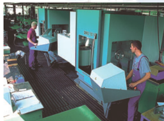
5 axis milling centers allow a production with high productivity even for small series and maximum working part sizes of 1,7 meter
