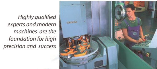
5 axis milling centers allow a production with high productivity even for small series and maximum working part sizes of 1,7 meter
