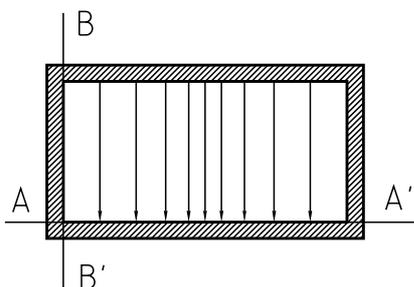
From these considerations it can be understood that at a given frequency a minimum size of one side of the rectangular waveguide is required to have the lowest order mode above cutoff. This minimum size is half the wavelength of the electromagnetic power. For a frequency of 2.45 GHz
