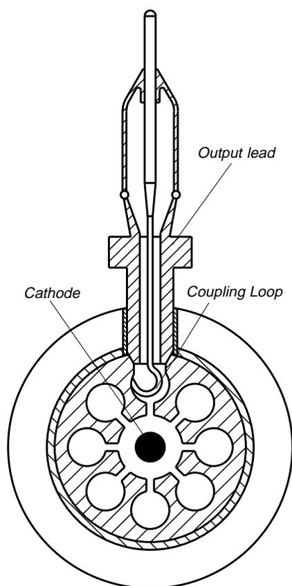
Cross Section of a Magnetron
